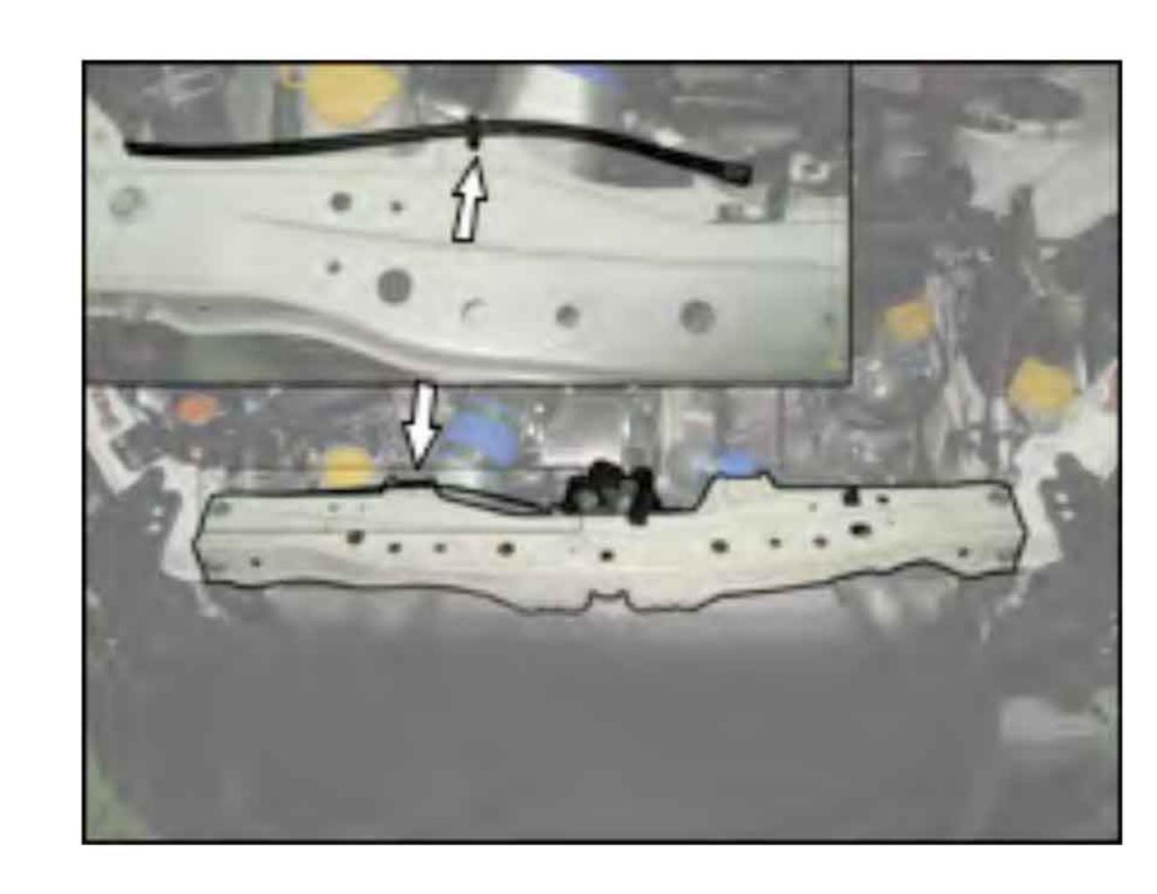
(2) Install the Intercooler Mounting Bracket Temporarily Finger Tighten.
