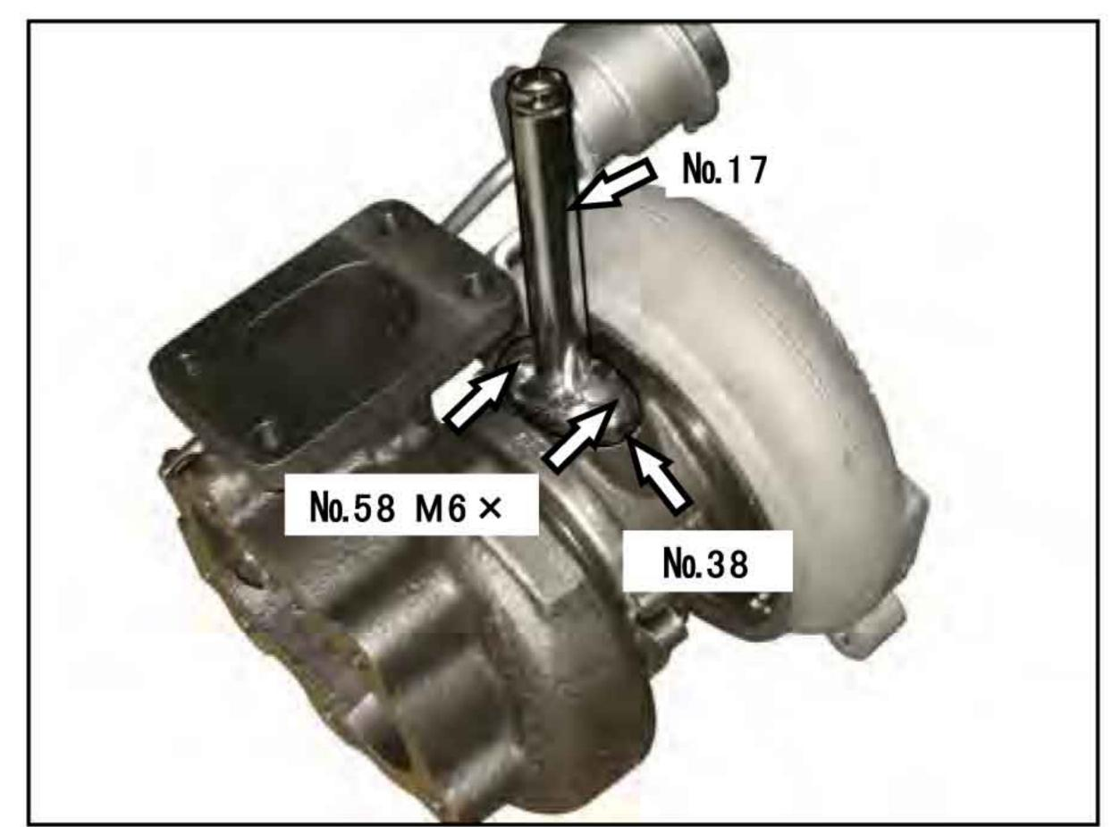
(4) Temporarily install the turbo and gaskets using the OEM bolts.
