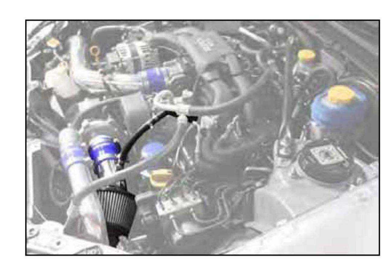
(3) Extend the ventilation hose using the 12mm hose union and supplied rubber hose. Connect the extended hose to the Air Intake Tube.
