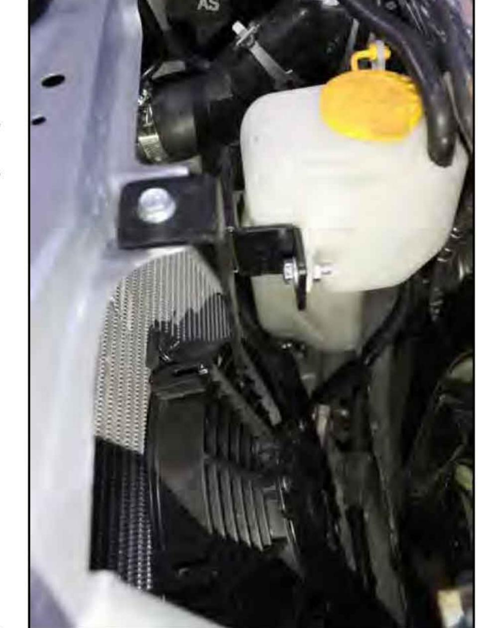
(4) Install reservoir tank brackets (Check with reservoir tank, reservoir tank brackets (Check with reservoir tank, then remove tank)
