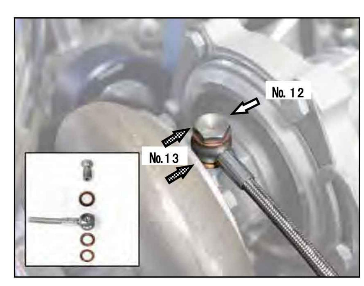
(6) Install the Oil Pressure Line between the Banjo Fitting and 90 degree elbow. Mount the Oil Pressure Line to the core support or upper radiator, using supplied Zip Ties.
