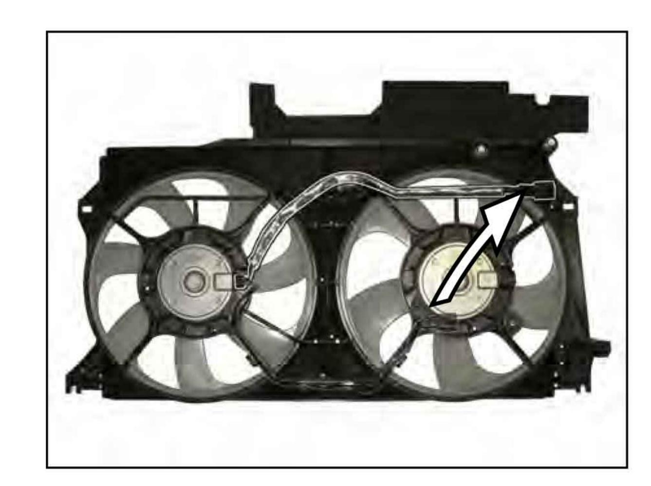
Change the location of the radiator fan harness and wrap with thermo wrap. thermo wrap.
