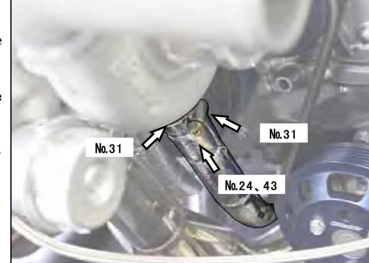
(2) Mount the Oil Return Hose to the Oil Return Hose Bracket. We recommend using stainless steel wire.
