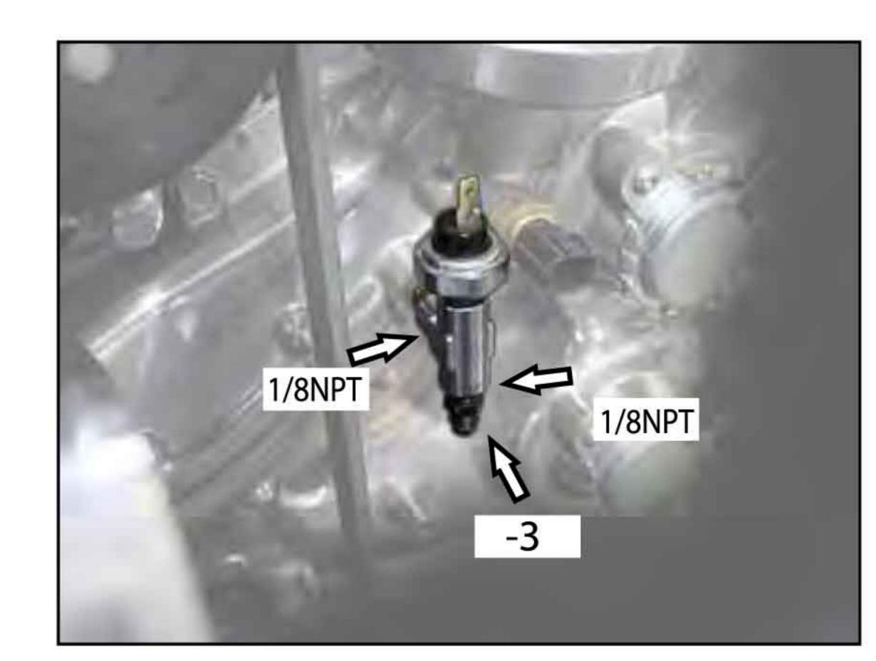
(4) Reconnect the Oil Pressure Switch Harness.
