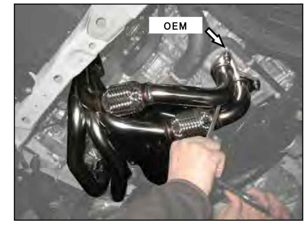
Install the oil return tube and gasket onto the turbo. ⟨Part # 1, 17, 38, 58⟩
